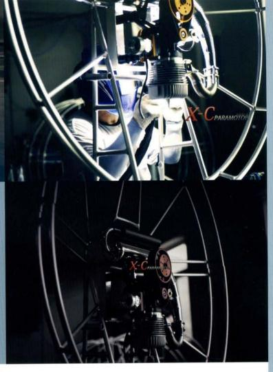
Frame is manufactured by aluminum alloy (Al6061). With flier centered design, disassembly and assembly are easy and transference is effortless. With light weight and minimum external shock, it will provide safe and comfortable flying experiences for all fliers.
